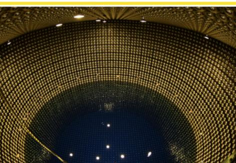
11,000 20" PMT inner detector 40% photo-coverage
