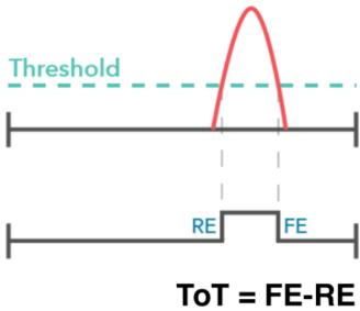
If several Rising Edges are recorded during the same T1, individual hit amplitudes are reconstructed using ToT
