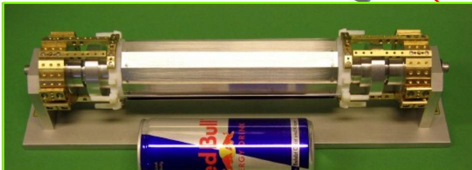
Mechanical mockup of pixel detector
