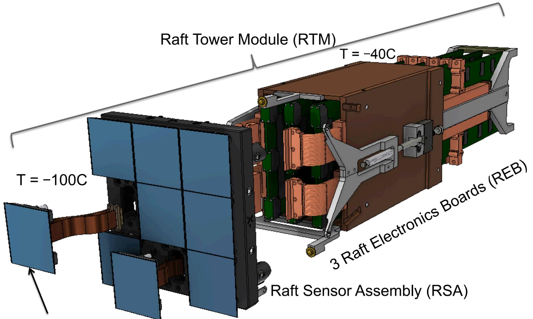
Individual sensor includes mechanical mount and flex cable
