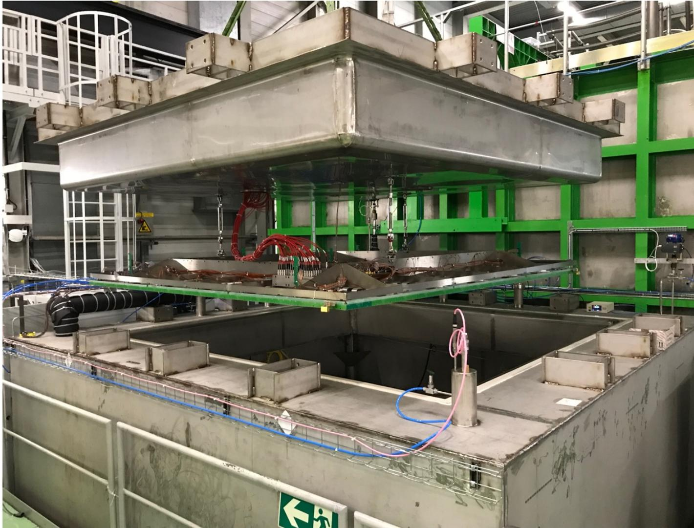
The cryo-vessel used to test the protoDUNE THGEMs will be modified and a full optical TPC will be instrumented
