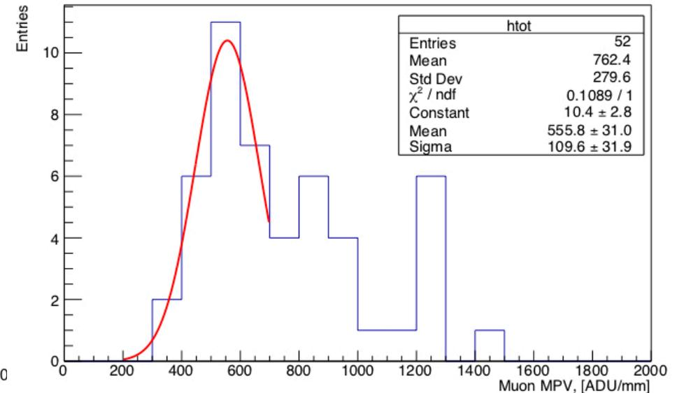
Distribution of MPV values for well fitted cosmic muon samples. Gaussian peak corresponds to the expected muon MPV energy loss of 1.6 MeV/cm.
