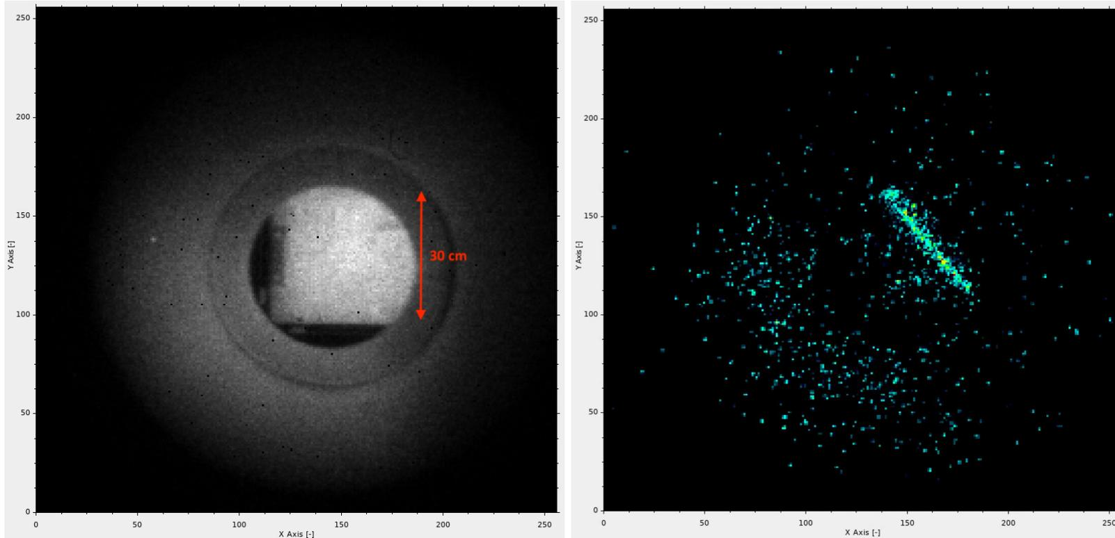
Left: Field of view seen when using the 11.5mm focal length lens (F/1.4). The 30cm x 30cm area that is visible of the THGEM only takes up roughly 1/4 of the total sensor area. The total field of view is approximately 1.2mx1.2m. The resolution is 4.5mm per pixel in x and y.
