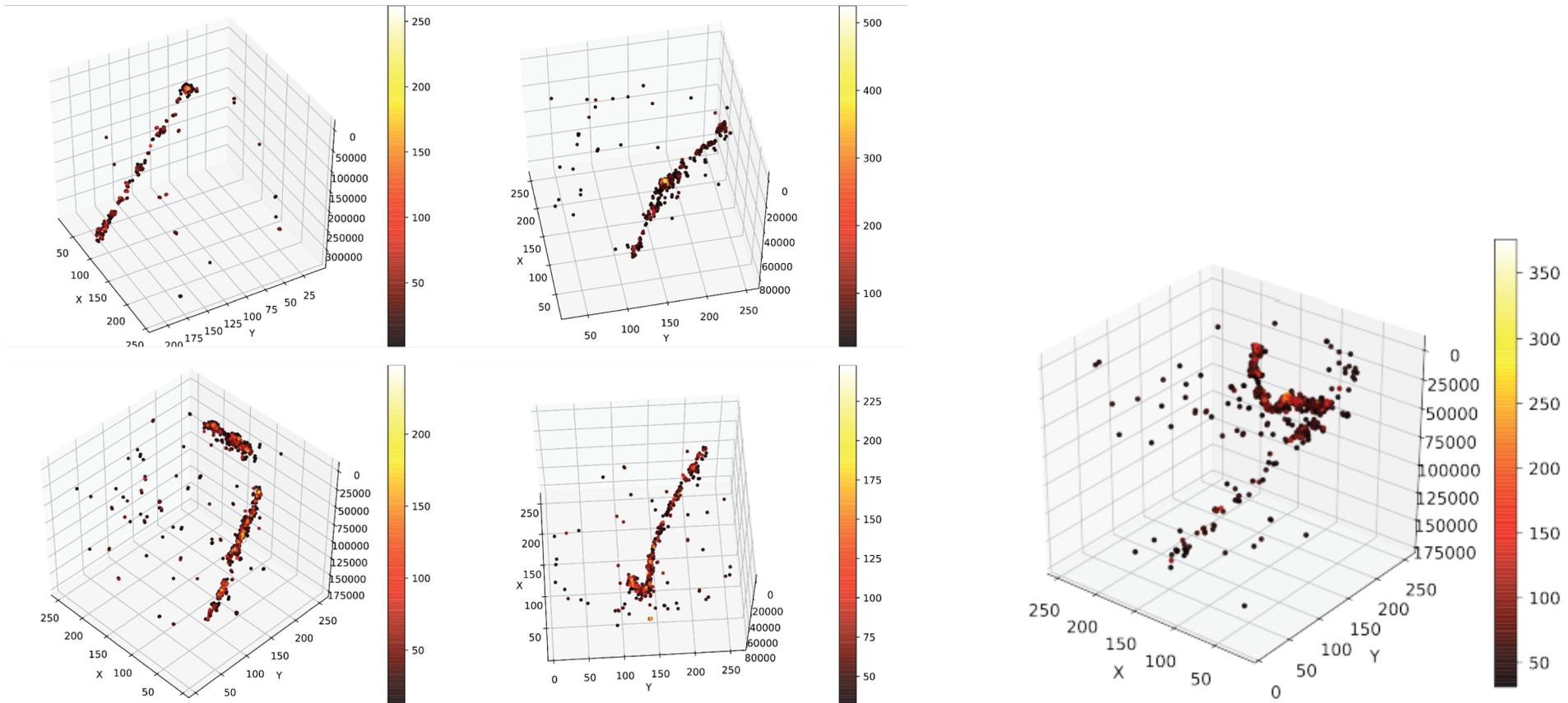
First demonstration of 3D optical readout of a TPC using a single photon sensitive Timepix3 based camera (<https://arxiv.org/abs/1810.09955>)
