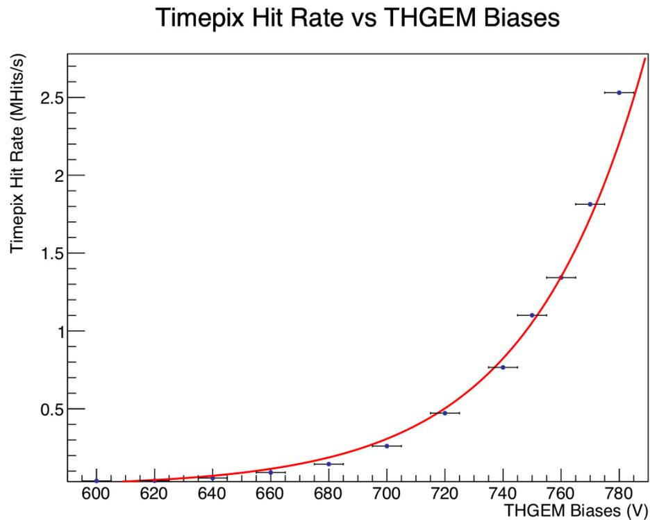
Camera pixel hit rate vs applied THGEM bias
