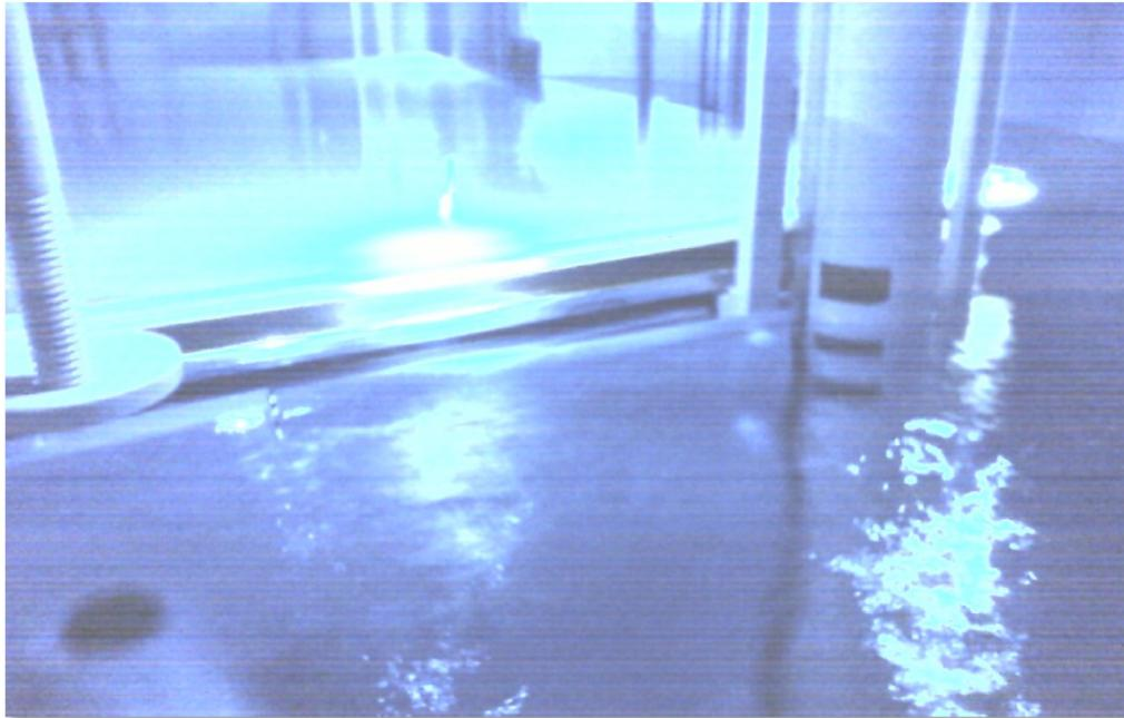
Cryogenic Monitoring Camera, viewing the THGEM at the liquid/gas interface
