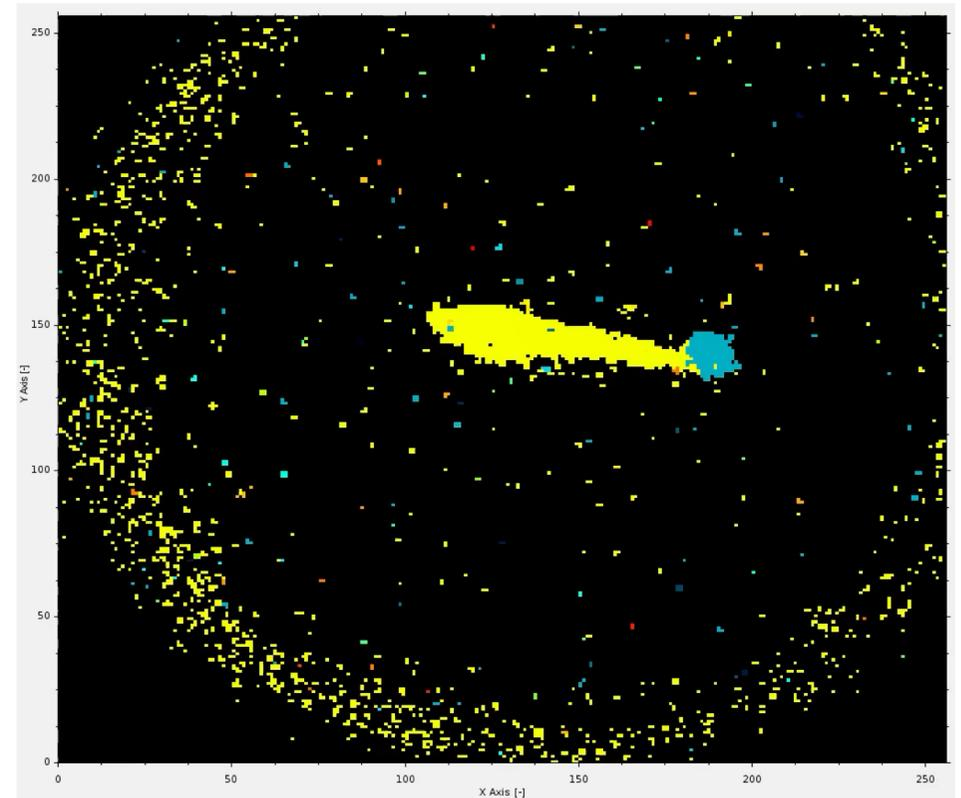
First demonstration of 3D optical readout of a TPC using a single photon sensitive Timepix3 based camera (<https://arxiv.org/abs/1810.09955>)
