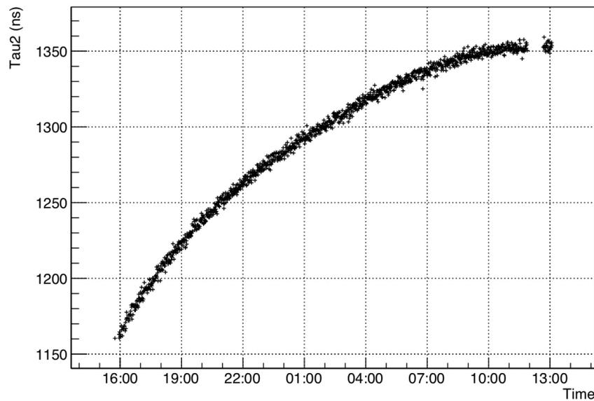
Sensitive to few ppb level, after that the electron lifetime needs to be calculated
