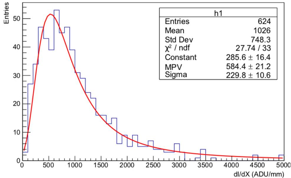
Sample distribution of summed hit intensities for 1 mm slices of a cosmic muon track.
