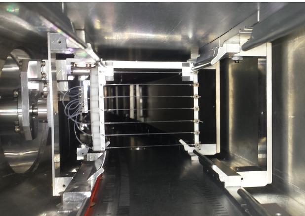
The fibre harps slide in to the beam to make a destructive measurement of the beam profile
