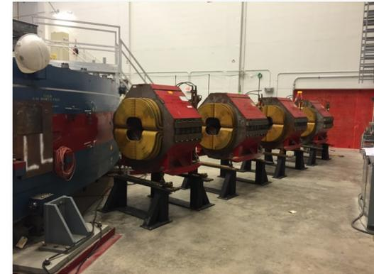
The kicker magnets provide a vertical magnetic field to put the muons on the correct orbit
